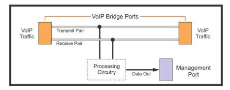
2 The Management Port is used to configured the device. Data is sent out this port to software applications that accept Caller ID via Ethernet. Connect this port to the same subnet that your Ethernet enabled Caller ID application is running.
